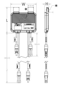
\*Clips can be removed for rack mounting Module frame specifications
